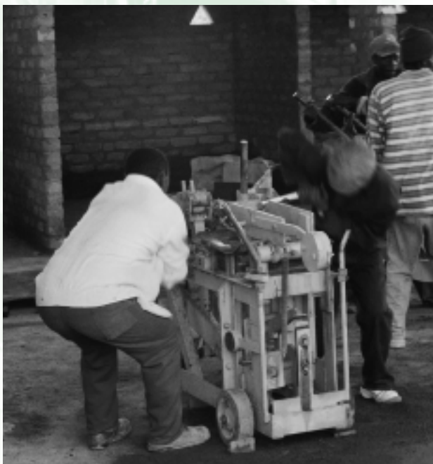
Fig. 2: Workers in cooperative making compressed earth blocks, Buffalo City, South Africa.
